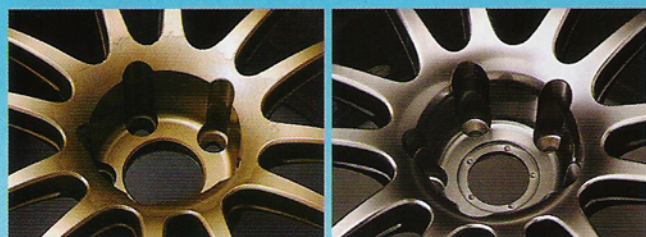
Diagram A: For the lightened version (Gold), the center cap area has been shaved down as you can clearly see the difference in diameter. Material has also been removed from the outer ring of the center area of the wheel increasing the diameter.
