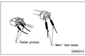
6) When checking continuity between connector terminals, or measuring voltage across the terminal and ground, always contact tester probe(s) on terminals from the wiring connection side. If the probe is too thick to gain access to the terminal, use "mini" test leads.
