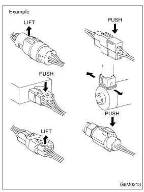
5) Some connectors are provided with a lock. One type of such a connector is disconnected by pushing the lock, and the other, by moving the lock up. In either type the lock shape must be identified before attempting to disconnect the connector.
