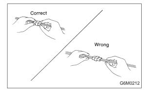
4) When disconnecting a connector, do not pull the wires, but pull while holding the connector body.
