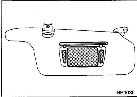
To use the vanity mirror, swing down the visor and open the cover. The lights beside the vanity mirror come on when the ignition switch is either in the "ACC" or "ON" position and the mirror cover is opened.
