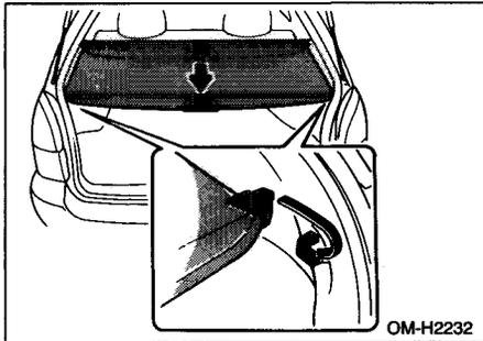
To extend the cover, pull the end of the cover out of the cover housing, then insert its hooks into the catches as shown. To rewind it, unhook it from the catches and it will rewind automatically.
