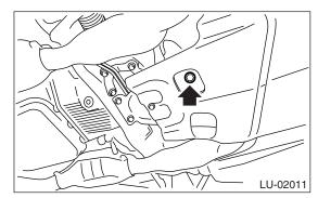
3) Tighten the engine oil drain plug after draining engine oil.
