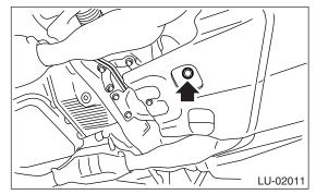
4) Fill engine oil through level gauge up to the center between upper level and lower level. Place the vehicle on a level surface when checking oil level. Use engine oil of proper quality and viscosity, selected in accordance with following.
